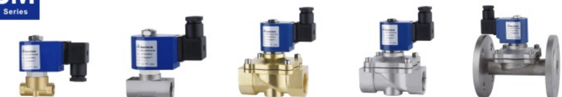
Body material: Forged Brass, SS Pipe size: 1/8"~2" Pressure: 0 ~ 55 kgf/cm 2 0 ~ 10 kgf/cm 2 Flange: DN15~25 Orifice: 4mm~7.5mm 16mm~50mm Fluid Media: Water, Hot Water, Air, Gas, Oil Etc.
