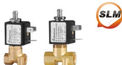
Body material: Brass Orifice: 1.5mm-2.5mm Pressure: 0-16kgf/cm 2 Pipe size: 1/8" -1/4"
