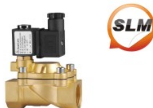
Body material: Brass Orifice: 12mm 20mm Pressure: 0.5-16kgf/cm 2 Pipe size: 3/8" -3/4"
