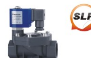
Body material: PA6 Orifice: 13mm ~ 40mm Fluid Media: Water, Hot Water, Air, Oil Etc. Pressure: 0.5 ~ 10 kgf/cm 2 Pipe size: 3/8"~1-1/2"
