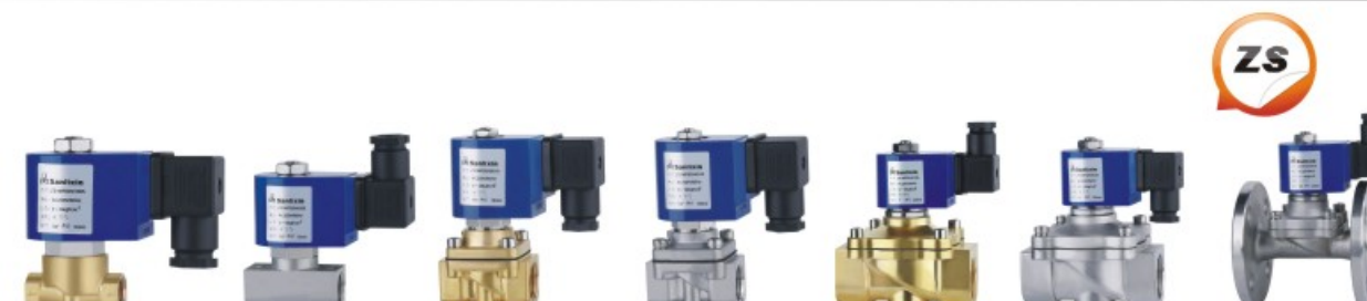
Body material: Forged Brass, Stainless Steel Pipe size: 1/8"~1" Flange: DN15~25 Pressure: 0 ~ 10 kgf/cm 2 0 ~ 20 kgf/cm 2 Orifice: 4.0mm~25mm Fluid Media: Water, Hot Water, Air, Gas, Oil Etc.
