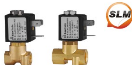
Body material: Brass Orifice: 1.0mm-2.5mm Pressure: 0-20kgf/cm 2 Pipe size: 1/8" -1/4"
